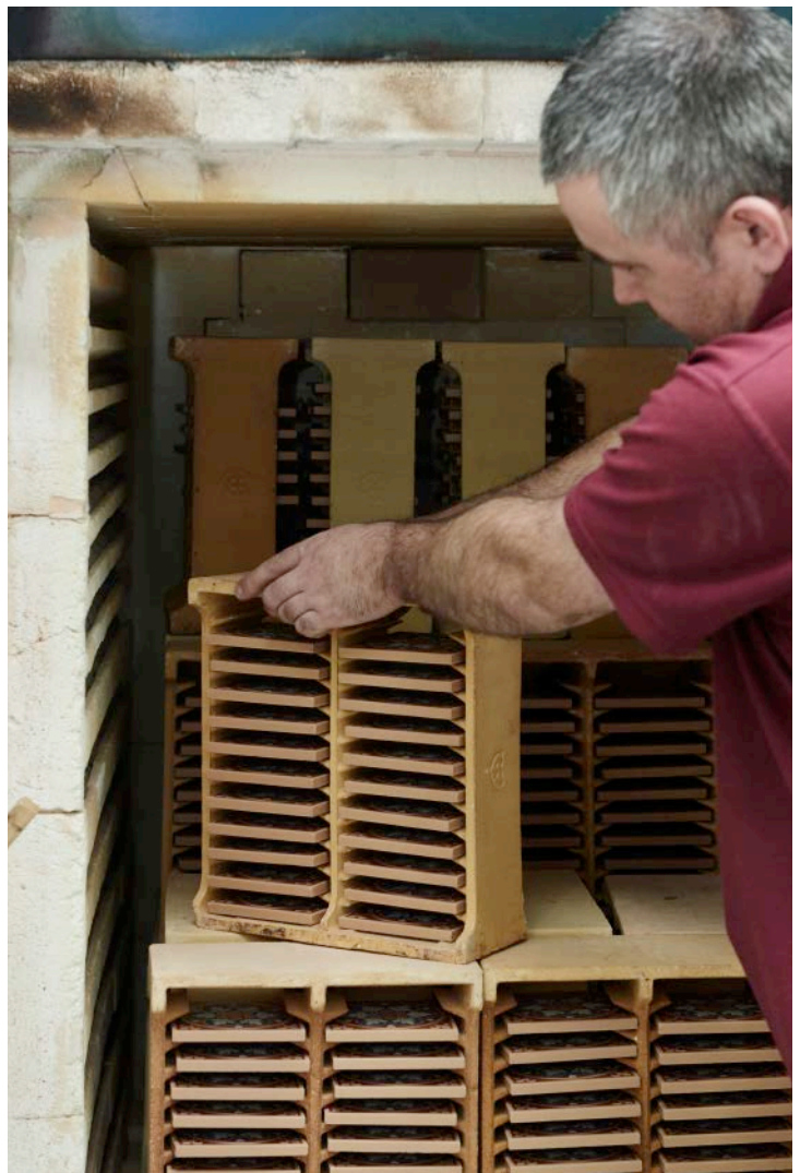
Front cover image: Oxford three colour pattern with modified Melville border in Chester Mews, Revival Grey and Dover White Above: Hand decoration and firing of Victorian Floor Tiles at our production facility in Exeter
